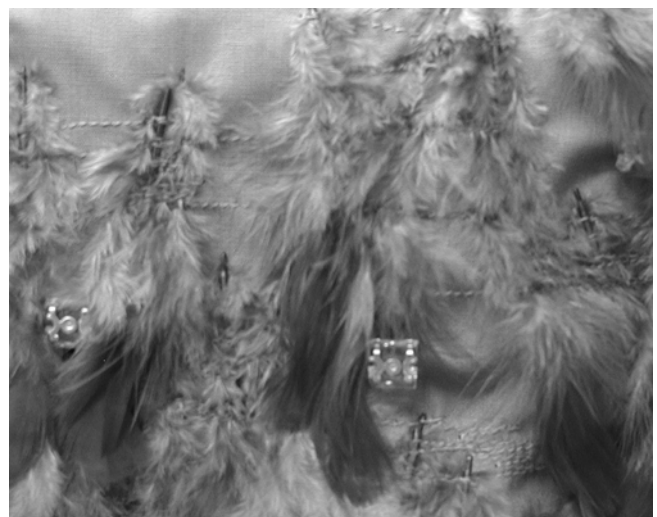
Figure 16. Light Emitting Diodes (LEDs) sewn into the feather surface with conductive yarns.
