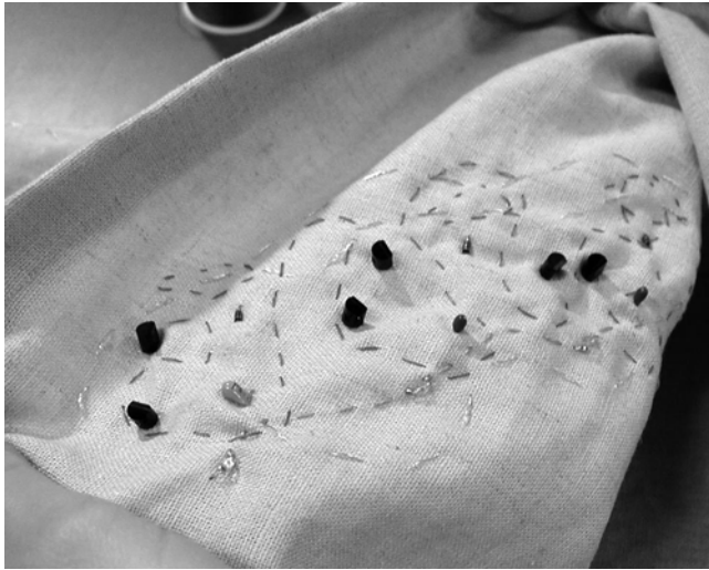
Figure 4. The soft circuit sewn into the Intimate Memory skirt
