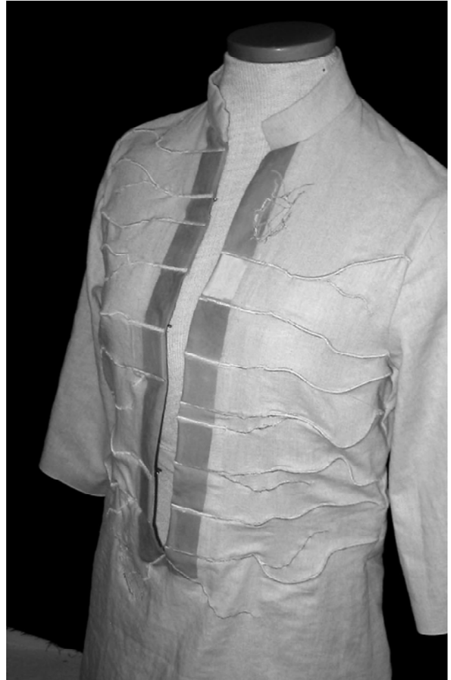
Figure 8. The Pure Play dress with thermochromic ink, Peltier junctions and stitched connections.
