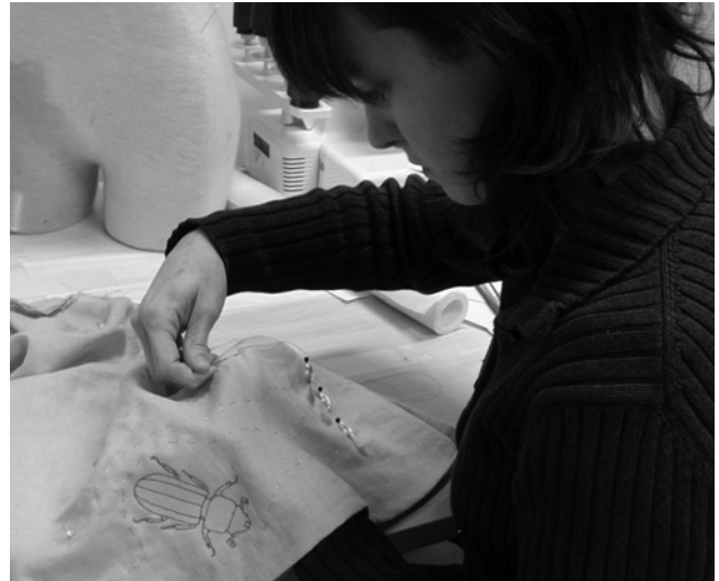
Figure 5. Stitching conductive thread into the Intimate Memory skirt
