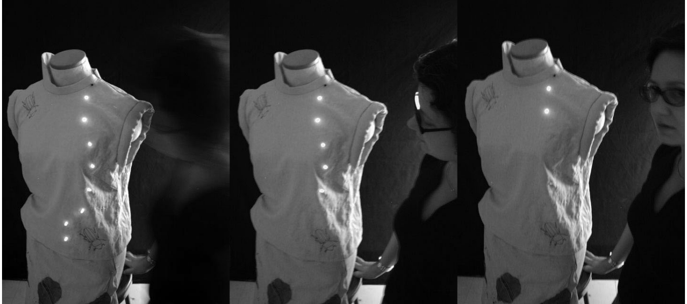
Figure 1. Intimate Memory shirt shows the time elapsed since the intimacy event occurred, by turning off LEDs one by one.
