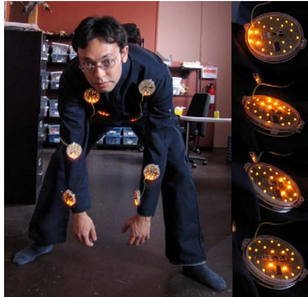
figure 3. Octopus modules distributed on the body and representation of motion and acceleration.
