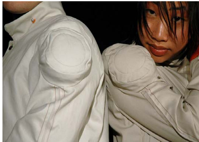
Figure 3. Detail of pockets that house electronic components and piping technique for the insulation of conductive threads.
