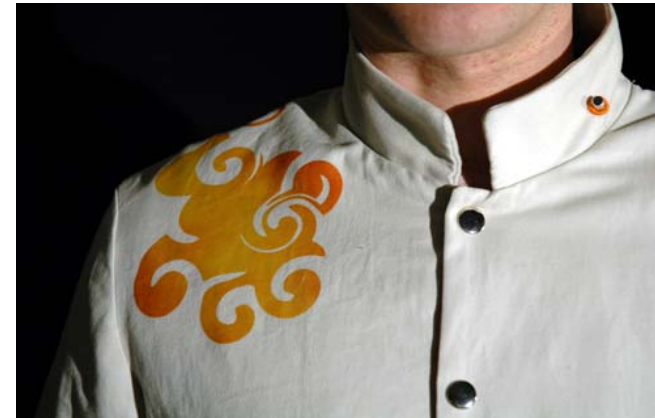
Figure 2. Shoulder patch of thermochromic ink and microphone integrated in the collar.
