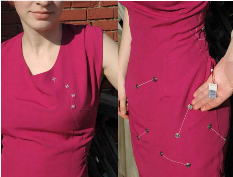
Figure 2. The electronic circuit is distributed over the body of the dress. The four LEDs provide the visual output. The power source consists of a lithium polymer rechargeable battery, held in a custom-made pocket at the waist. The interactive interface consists of the pairs of snaps that act as switches and allow us to close the circuit (turn the LEDs on) by connecting to another dress.
