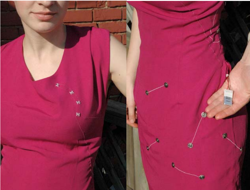
Figure 2. The electronic circuit is distributed over the body of the dress. The four LEDs provide the visual output. The power source consists of a lithium polymer rechargeable battery, held in a custom-made pocket at the waist. The interactive interface consists of the pairs of snaps that act as switches and allow us to close the circuit (turn the LEDs on) by connecting to another dress.
