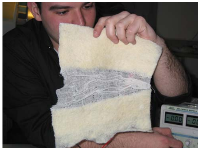
Figure 5: Marcelo connects the power supply to the woven sample and watches it contract. Photo by Tracey Doyle.
