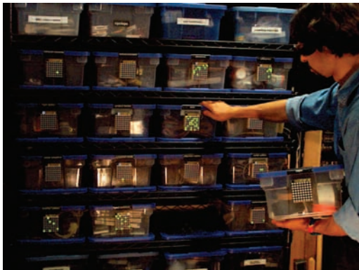
Figure 8 TouchCounters showing correlation of usage of multiple containers.
