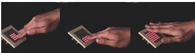
Figure 9 FishFace electric field sensing modules for non-contact, gestural input.
